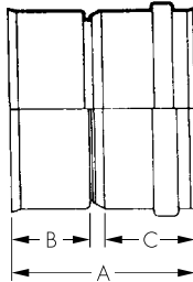
Adaptor (double socket) twinwall to solid-wall PVC-U pipe
