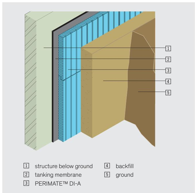
Figure 1: Principles of insulating structure below ground
