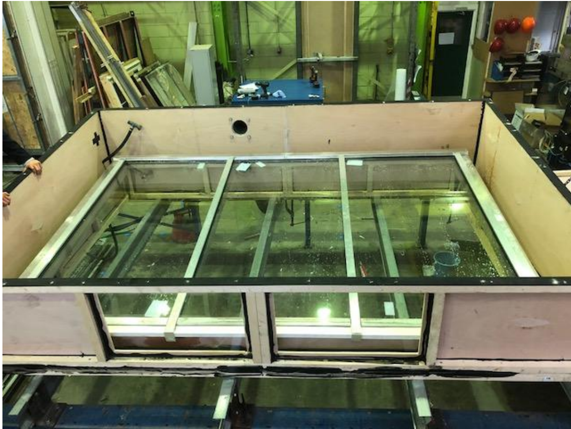
Figure A1. Lonsdale Metal Inclined Rooflight installed in airtight box on BREs ACR Rig
