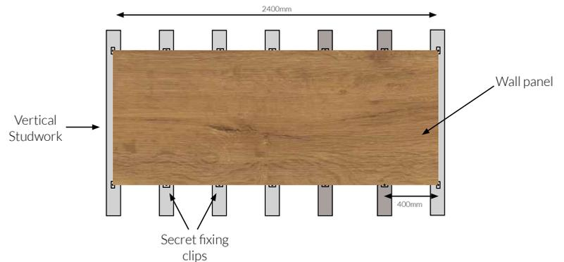
The panels can be fixed to metal or timber vertical/horizontal studwork at 400mm centres, blockwork or other suitable substrates after the black fleece has been installed.
