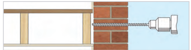
1. Mark the position of the joist centre on the external wall and then drill a clearance hole (normally 16mm) through the wall. Clean out the hole
