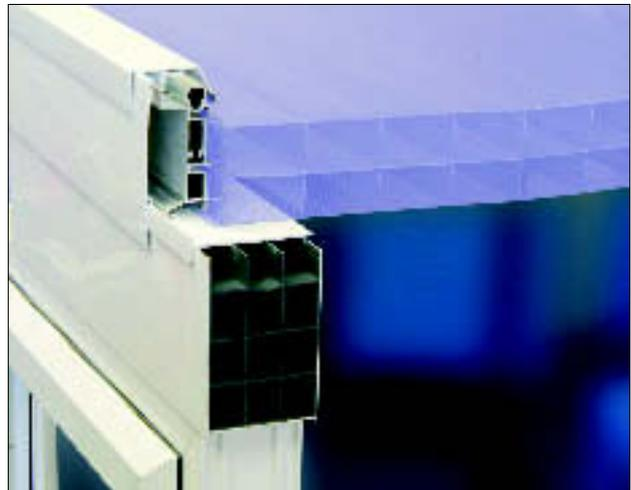
9.5 The PVC-U eaves closure trim is then fitted followed by the PVC-U gable end trims and external PVC-U glazing bar cappings with co-extruded TPE gaskets. The glazing bar cappings are clipped onto the glazing bars to form a seal against the glazing panel.
