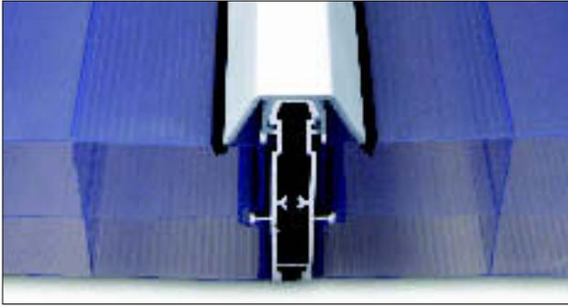
1.6 The glazing panels are joined together by aluminium glazing bar sections extruded from aluminium to BS EN 755-2 : 1997<sup>(1)</sup>, material designation 6063-T6, with PVC-U external claddings with TPE co-extruded gaskets.
