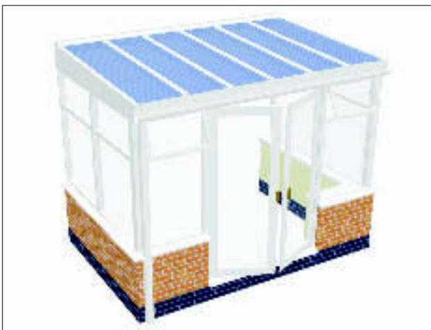
1.3 This Certificate relates to roofs up to 3.5 m spans used anywhere in the UK and up to 4 m spans where the negative wind pressure does not exceed 0.75 kNm<sup>-2</sup>. Within these parameters, the
