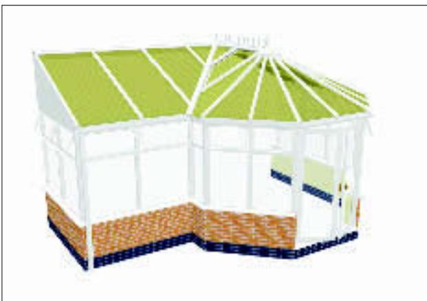
1.5 The roof system (see Figure 6) consists of a ridge beam member and glazing bar sections extruded from aluminium to BS EN 755-2 : 1997<sup>(1)</sup>, material designation 6063-T6, glazed with three or five wall polycarbonate panels of either 16 mm, 25 mm or 32 mm thicknesses or 24 mm double-glazed sealed units that carry the BSI Kitemark to BS 5713 : 1979. An aluminium ring beam is attached to the supporting side wall
