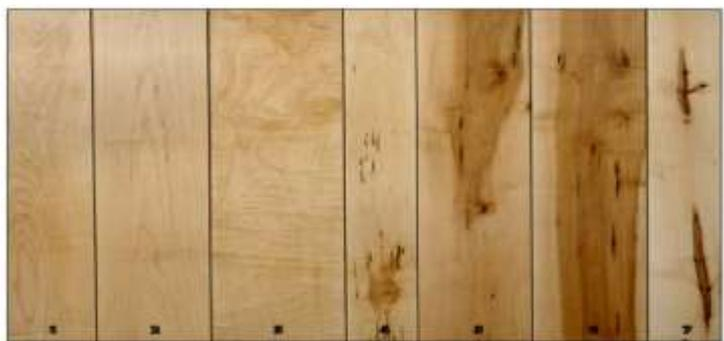
The picture to the right shows the boards cut from a single tree we will only use the first two (1 & 2) boards to manufacture our Prime Hard Canadian Maple Engineered Flooring. Sometimes we will include board 3 but the rest with mineral defects we use elsewhere.
