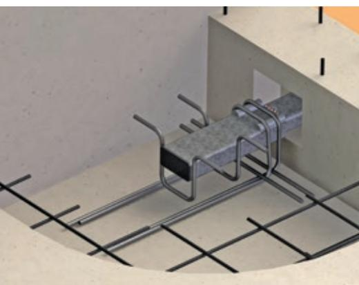
Figure 9: View of a TSS telescopic insert.
