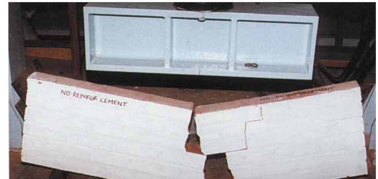
Destruction testing of un-reinforced wall
