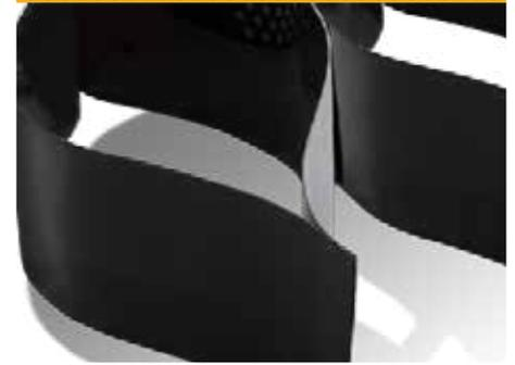
ABG manufacture Erosaweb as a three dimensional geocell system developed for top soil/stone retention on steep railway embankment slopes. Once installed it forms a blanket of shallow pockets across the slope face into which fill is placed. Once filled, it protects the slope and fill from erosion forces whilst allowing vegetation to establish for long-term protection.
