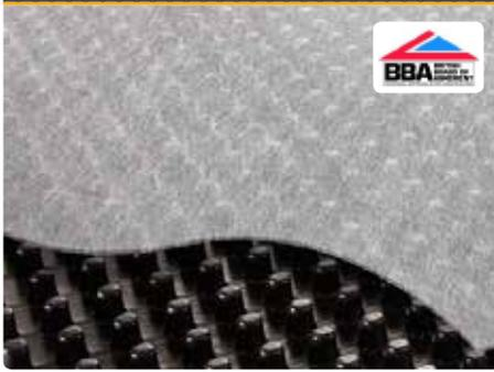
ABG manufacture Deckdrain as a high performance drainage and protection layer for relief of hydrostatic pressure from buried structures such as bridge abutments, retaining walls, culverts, basements, cut & cover tunnels, etc.
