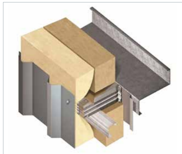
Standard fire wall construction using glass fibre to the external side of the Ashgrid bar and rock wool to the internal side. Both layers are trapped by the spacer system. Provides 4 hour stability and 30 mins insulation. Where both layers are used as glass fibre it will provide 15 mins insulation timing. For all fire walls installers, detailers and specifiers must refer to our full reports.
