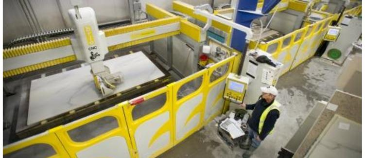
*CNC Equipped Stone Cutting Machinery*
