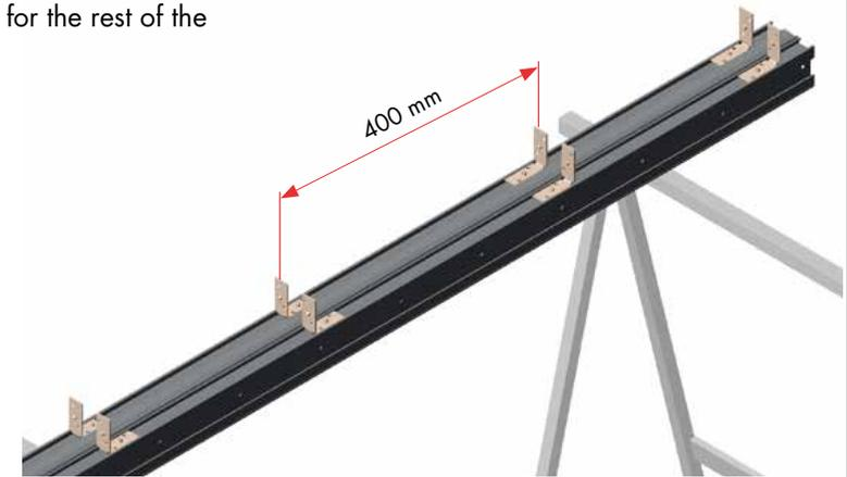
6. Attach UPM ProFi Quiet Tape into the designated top grooves of the support rails.
